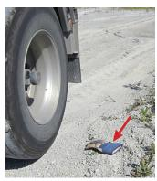
Drivers can create their own landmark by placing a glove on the ground at the first point they want to back to.
