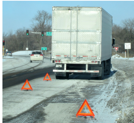
This driver did not set his triangles out correctly. See diagrams below for proper placement.
